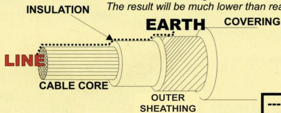
With Guard Connected, Surface Leakage Current is eliminated by the Guard Test Lead. Therefore eliminating measurement error. The result will be correct.
