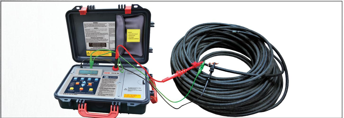
Without Guard Connection, Error Surface Leakage Current Circulate between Line and Earth Test Probes, creating a measurement error. The result will be much lower than real.
